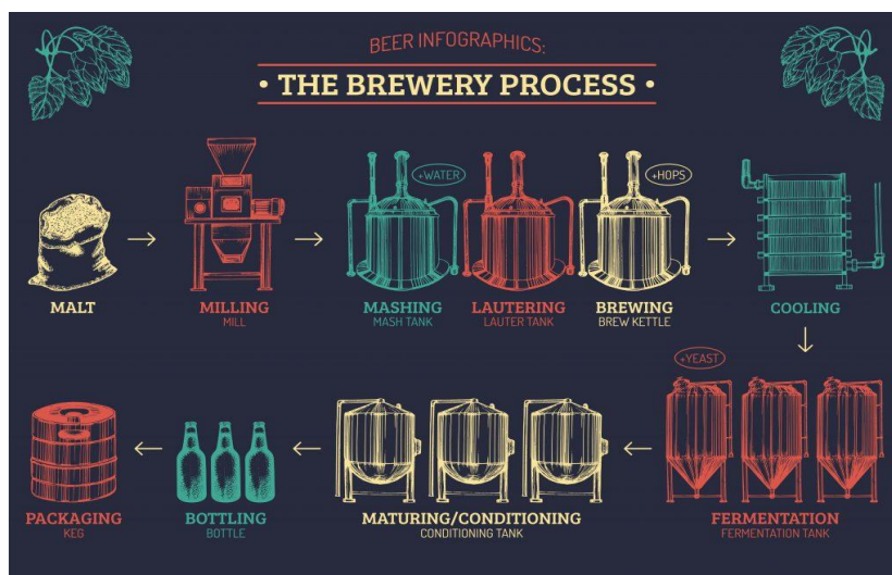
Fig -2: A flow diagram showing the main steps in the creation of industrial beer
