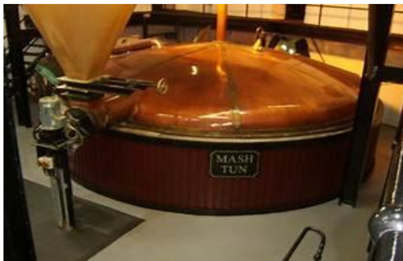
Fig -4: Industrial mash tun used for enzymatic conversion of malt starch into fermentable wort
